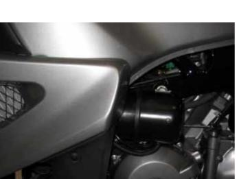
The **Cable Interface Unit (5)** is mounted on the ECU bracket on the left side. It has a new **cable (6)** running from it to the throttle bodies.
